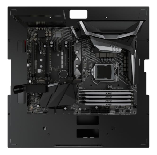
Maximum: <305 x280mm SSI-CEB Minimum : ATX Motherboard
